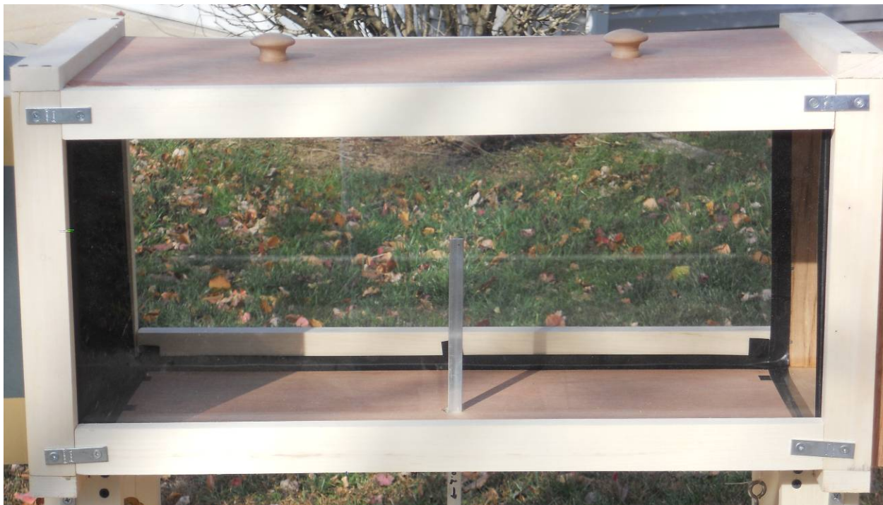
Figure 8. Test section with Plexiglas ® sides and plywood top and bottom.
