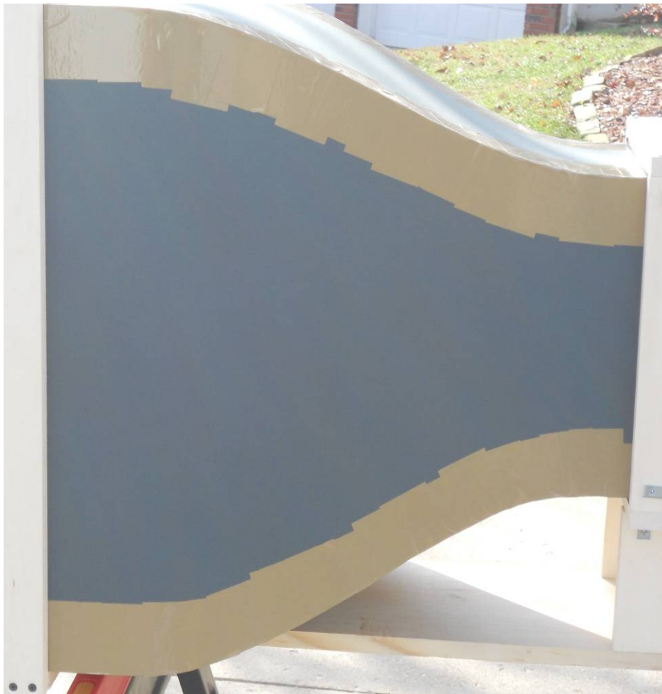
Figure 6. Side view of contraction made of mat board.
