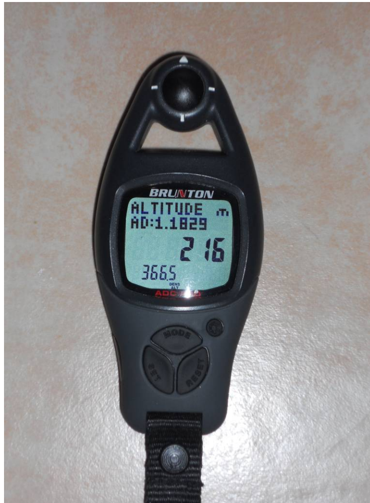
Figure 12. Brunton ADC Pro used for validation experiments and to routinely measure air density.
