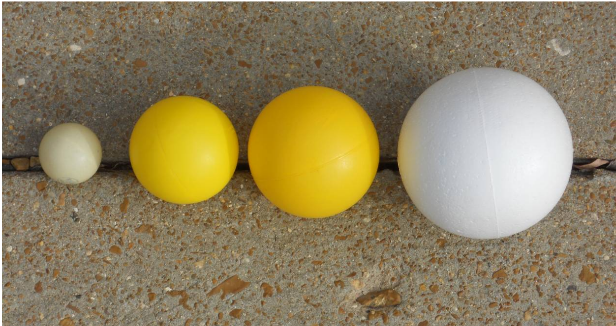
Figure 16. Balls used to calibrate/validate wind tunnel.
