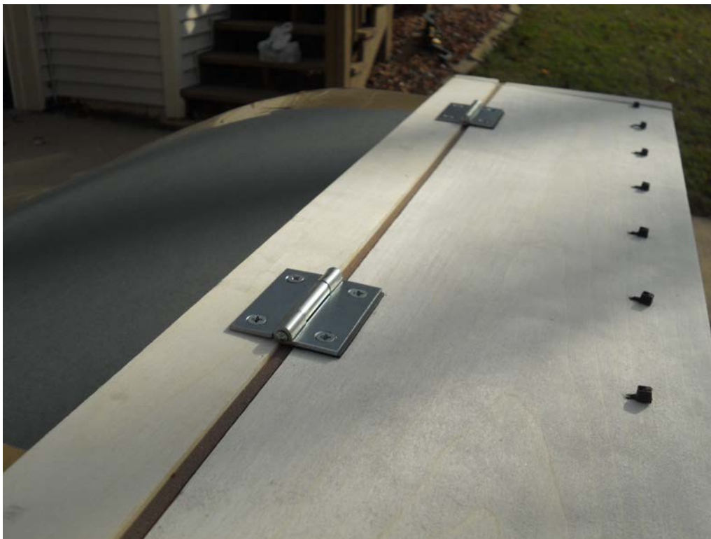
Figure 5. Hinges attaching the inlet/settling chamber to the front of the contraction.
