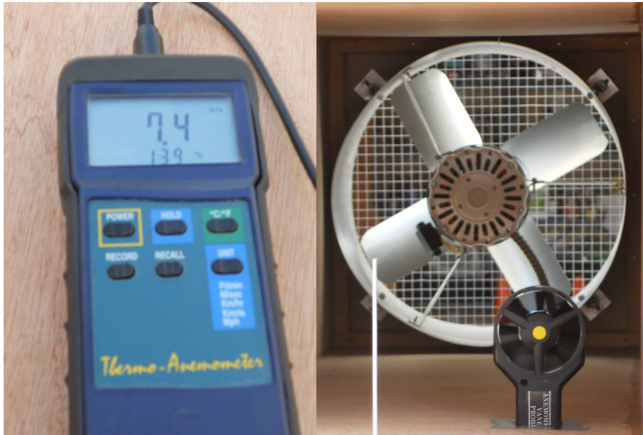
Figure 11. Exetech anemometer used to measure wind tunnel speed.
