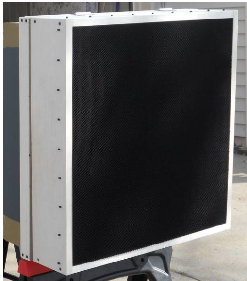
Figure 2: View of front of wind tunnel showing black plastic honeycomb.
